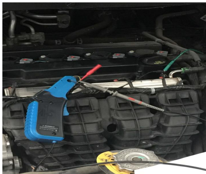
Pic-3 use of current clamp
